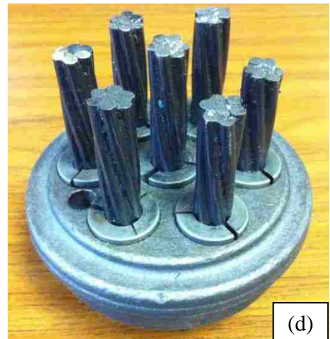
Figure 3-9 Anchor head components: (a) complete assembly; (b) strand wedge; (c) wedge plate; and, (d) seated strands
