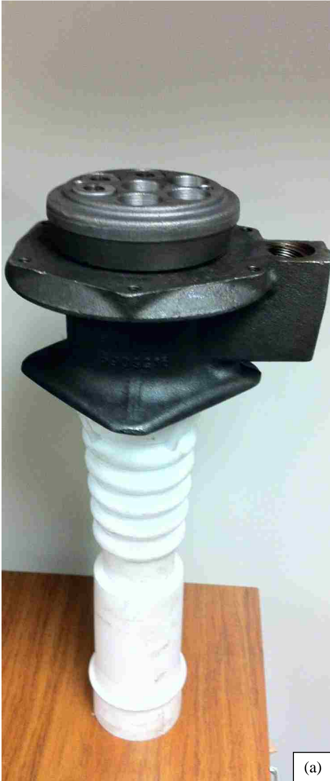
Figure 3-9 Anchor head components: (a) complete assembly; (b) strand wedge; (c) wedge plate; and, (d) seated strands
